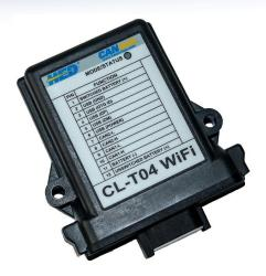
The CL-T04 is a solid-state microprocessor based module and member of the HED® CANLink® multiplexed control family. Delivered in a Deutsch enclosure, this unit provides a WiFi wireless interface.
