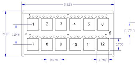
Do not mount keypad in way that will seal/block/plug the vent hole, preventing gore vent from breathing.
