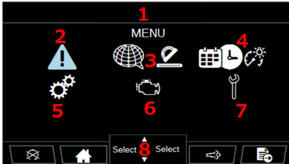
6. Engine Type selection – has no effect on operation of the display. Type is set in the chart
