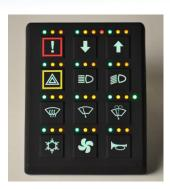
The HED® CL-608 is a solid-state microprocessor based keypad module that is a member of the HED® CANLink® multiplex control family. It provides a versatile, programmable, and highly visible operator interface.
