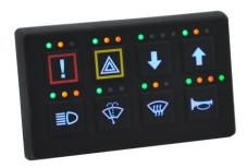
The HED® CL-610 is a solid-state microprocessor based keypad module that is a member of the HED® CANLink® multiplex control family. It provides a versatile, programmable, and highly visible operator interface.
